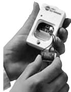
The battery can be changed using the battery set (item no. 0515.0019) which is available as an accessory.
